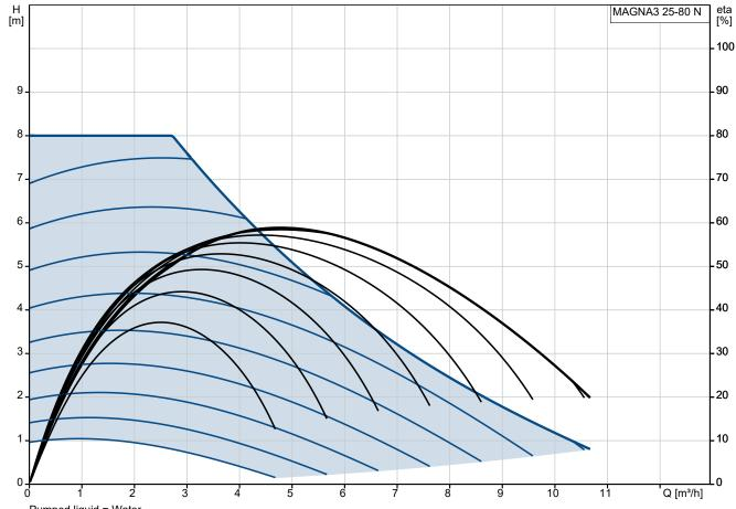
Pumped liquid = Water Liquid temperature during operation =  $60 \, ^{\circ}$ C Density =  $983.2 \, \text{kg/m}^3$
