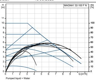
Pumped liquid = Water Liquid temperature during operation = 60 °C Density = 983.2 kg/m³
