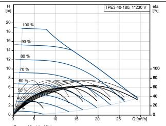
Pumped liquid = Water Liquid temperature during operation = 20  $^{\circ}$ C Density = 998.2 kg/m³
