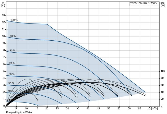
Liquid temperature during operation = 20 °C
