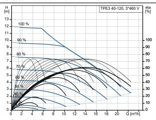
Pumped liquid = Water Liquid temperature during operation = 20  $^{\circ}$ C Density = 998.2 kg/m³
