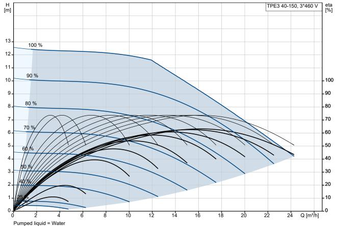
Liquid temperature during operation = 20 °C
