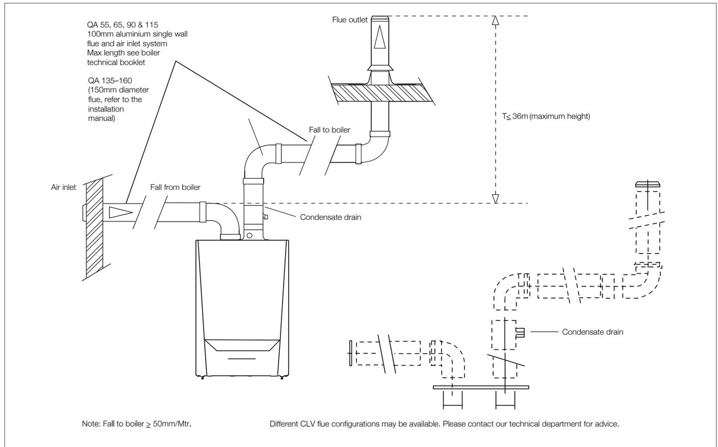
**Note 1:** Fall to boiler  $\geq 50\text{mm/Mtr.}$
