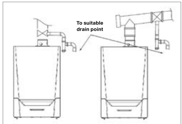
**Note:** The condensate trap should be as close as practical to the condensate outlet and the trap and pipework should be adequately supported.
