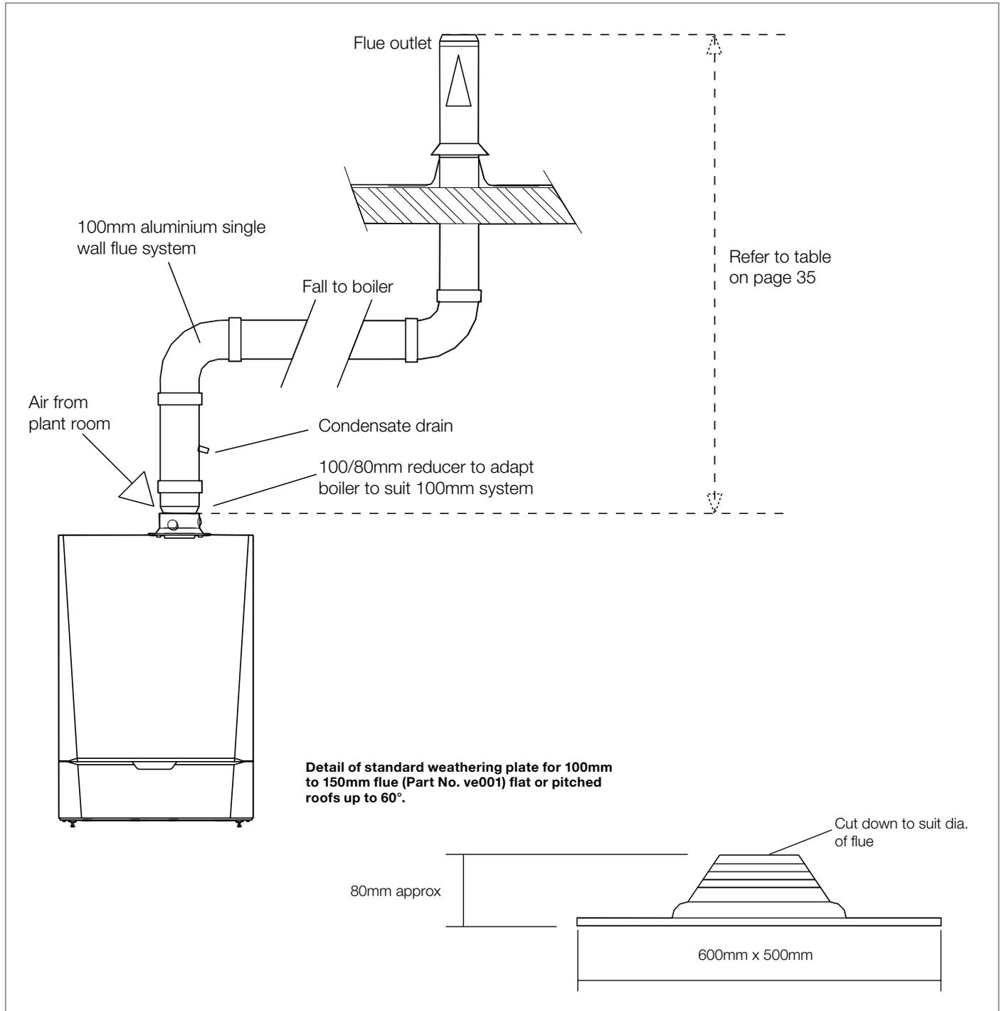
**Note:** Fall to boiler  $\geq 50\text{mm/Mtr.}$
