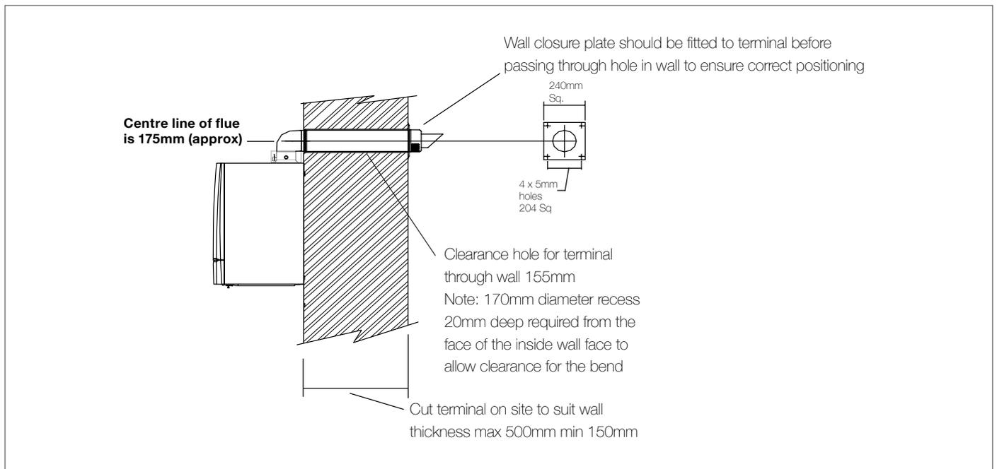
**Note 1:** Fall to boiler  $\geq$  50mm/Mtr. **Note 2:** Boiler bend and wall plate are included.
