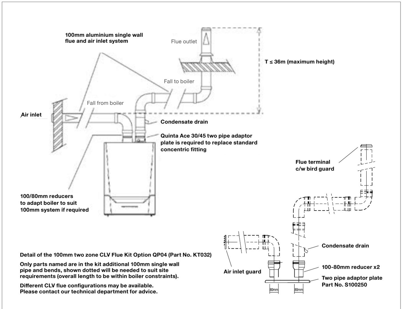
**Note 1:** Maximum combined length of air intake and flue is 40m.
