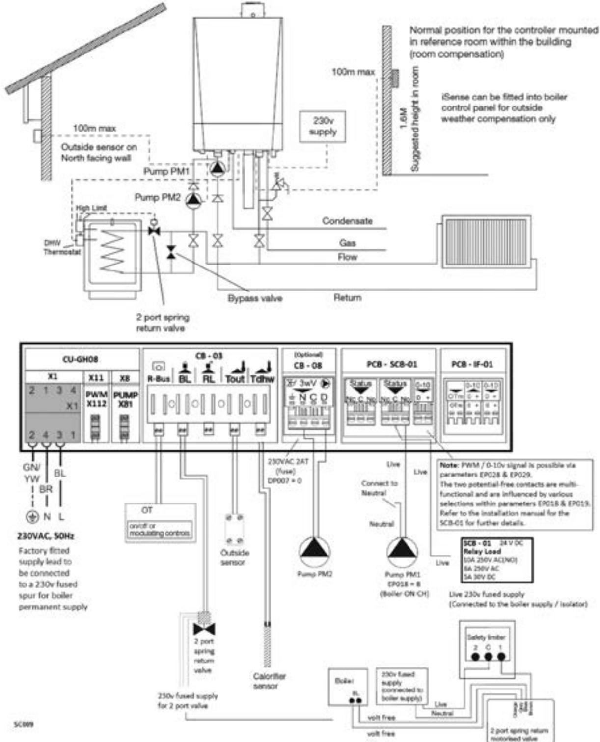
**Note:** When using the Remeha supplied low loss header and pump kit and the DHW diverting valve or primary pump kit, the calorifier must be sited within 3m of the boiler. In both cases, the DHW cylinder must be a high recovery unit capable of accepting the full or adjusted DHW output of the boiler used. Control PCBs are shown diagrammatically. Earths are omitted for clarity.
