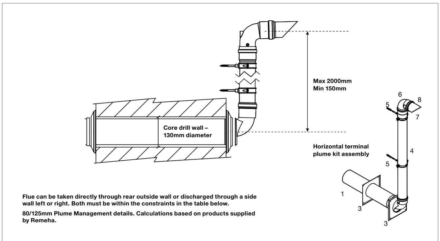
**Note 1:** Both the concentric flue terminal and plume flue outlet positions of the Plume Management Kit (PMK) must comply with the current regulations and British Standards with regards to the minimum distances from openings, walls, etc.
