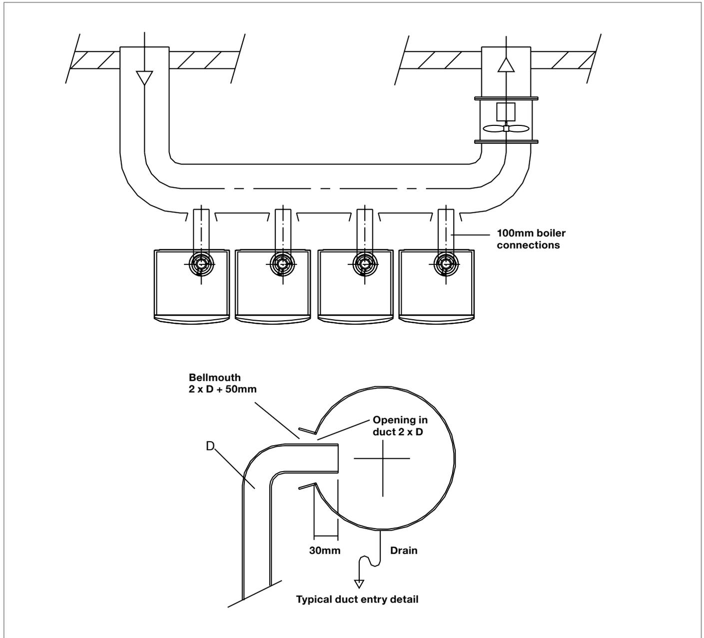
For illustration purposes only (we recommend installation of condensate collectors with drainage system and water sealed siphon to the spigot of each boiler).
