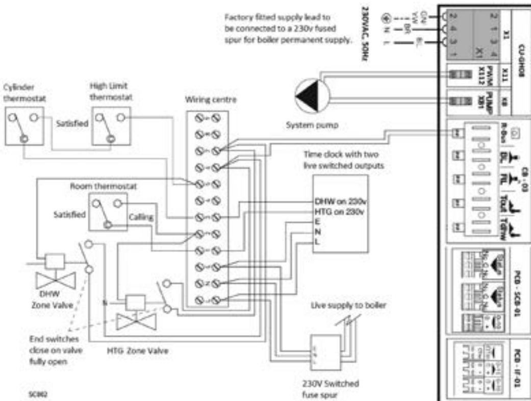
**Note:** Control PCBs are shown diagrammatically. Earths are omitted for clarity.
