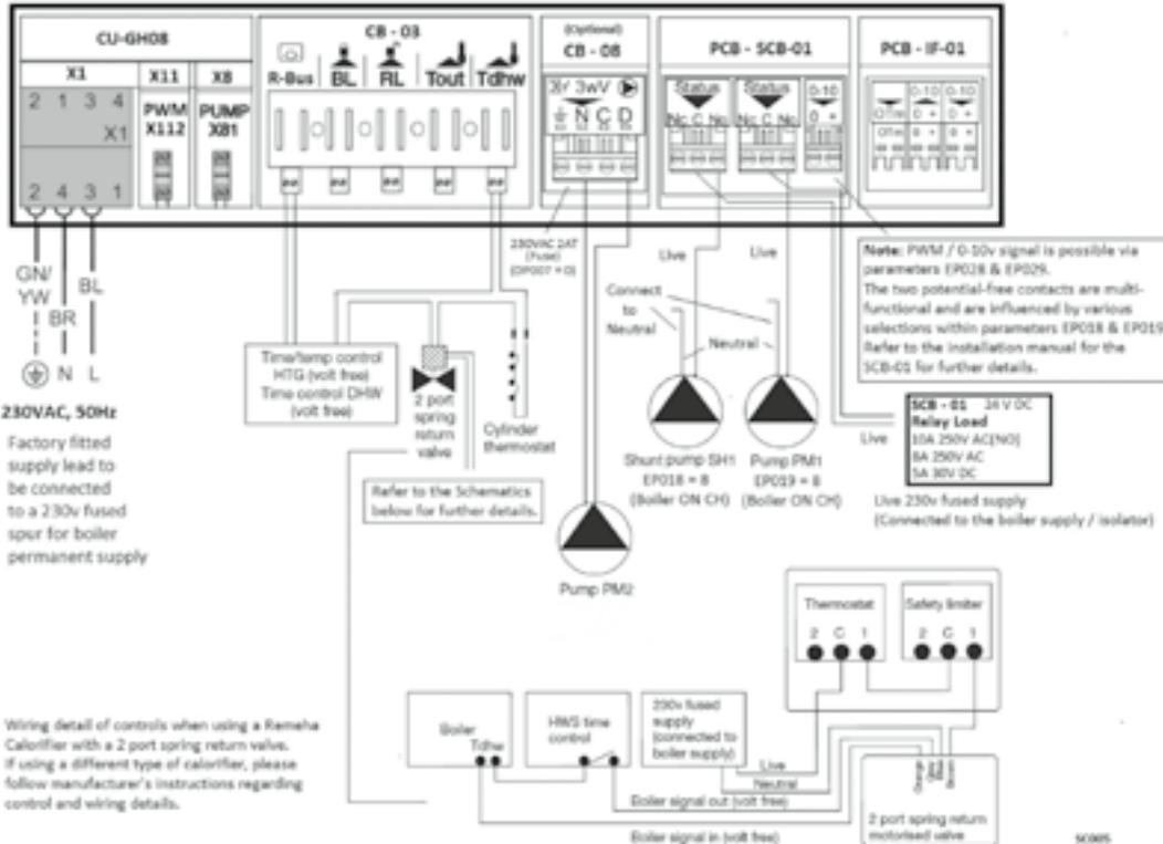
**Note:** When using the Remeha supplied low loss header and pump kit and the DHW diverting valve or primary pump kit, the calorifier must be sited within 3m of the boiler. In both cases, the DHW cylinder must be a high recovery unit capable of accepting the full or adjusted DHW output of the boiler used. Control PCBs are shown diagrammatically. Earths are omitted for clarity.
