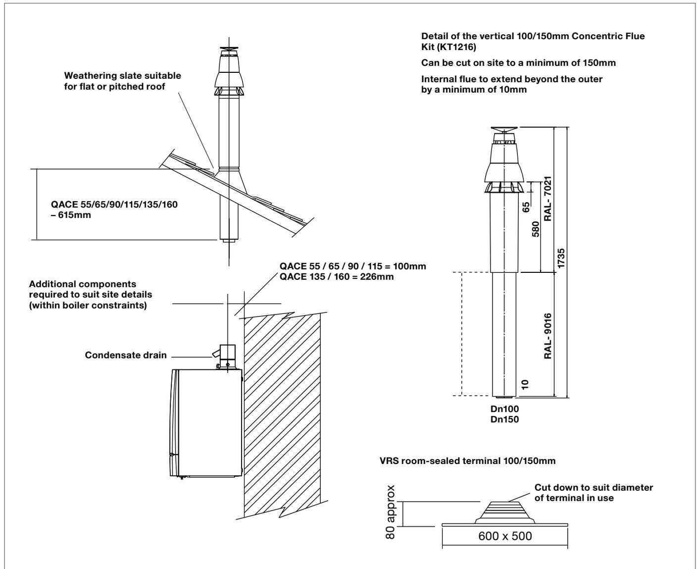
**Note:** It is recommended a condensate drain is used for vertical flue lengths above 1.5m.
