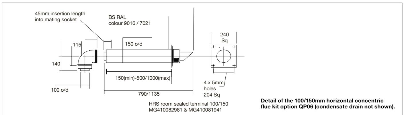
**Note 3:** All dimensions are in mm. **Note 4:** Boiler bend and wall plate are included.
