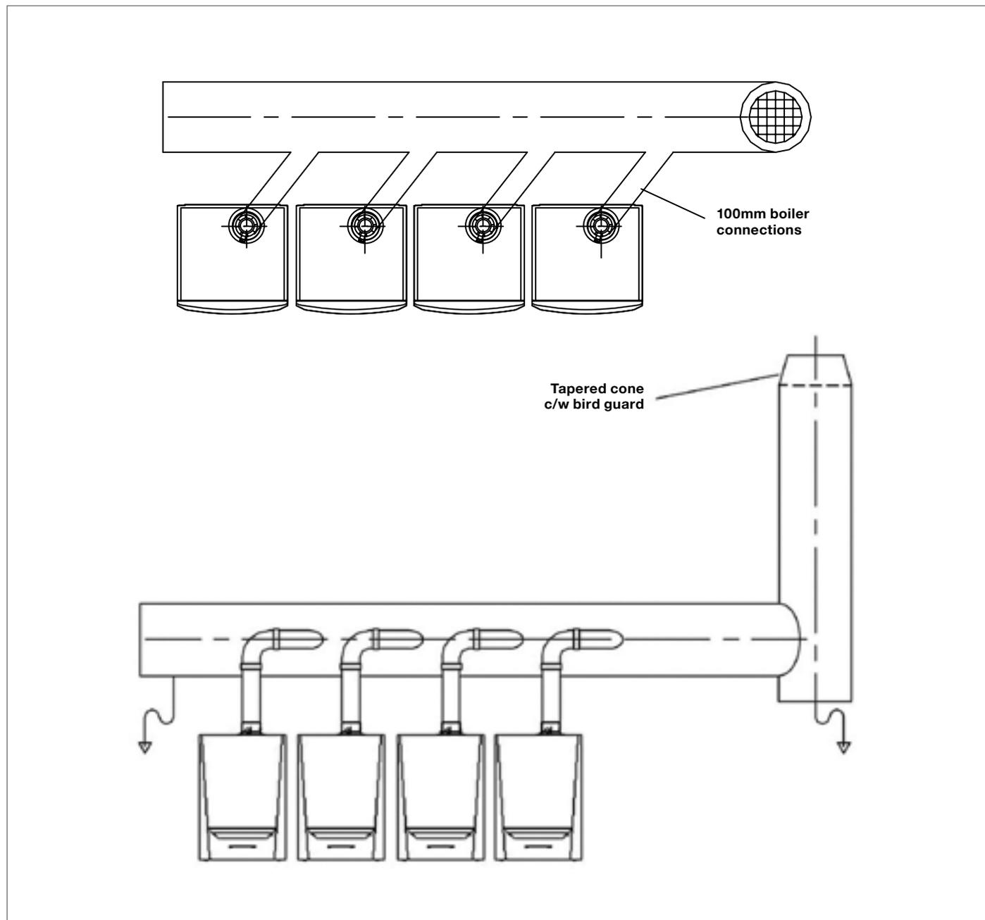
For illustration purposes only (we recommend installation of condensate collectors with drainage system and water sealed siphon to the spigot of each boiler).
