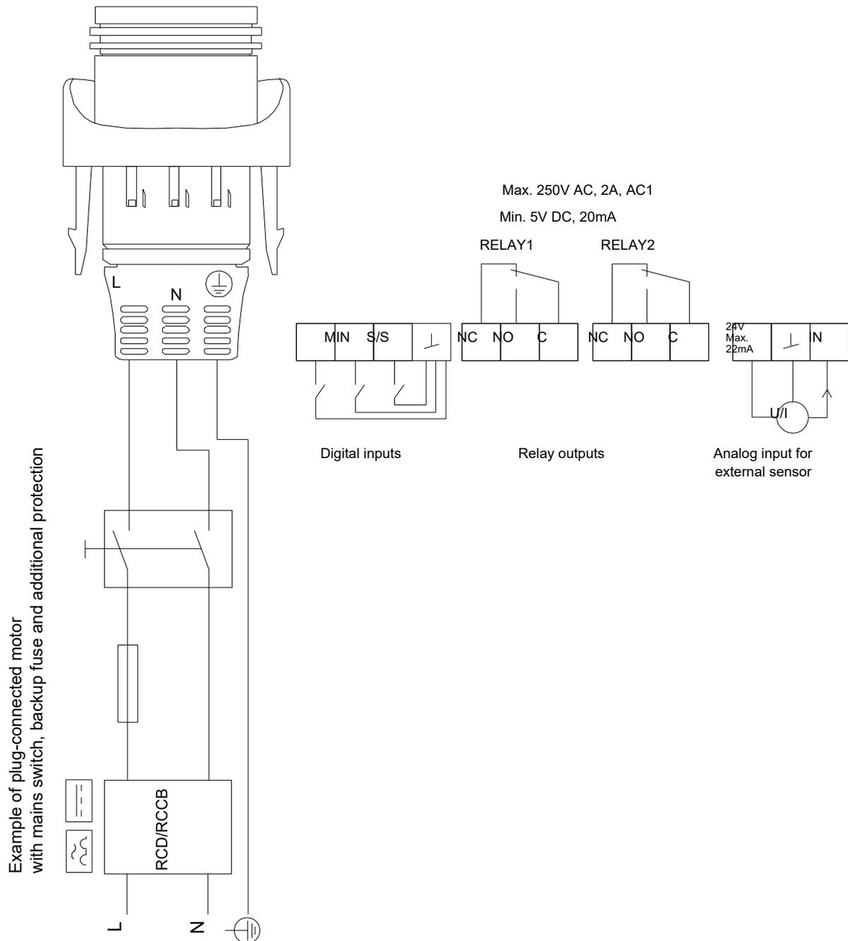
Example of plug-connected motor with mains switch, backup fuse and additional protection
