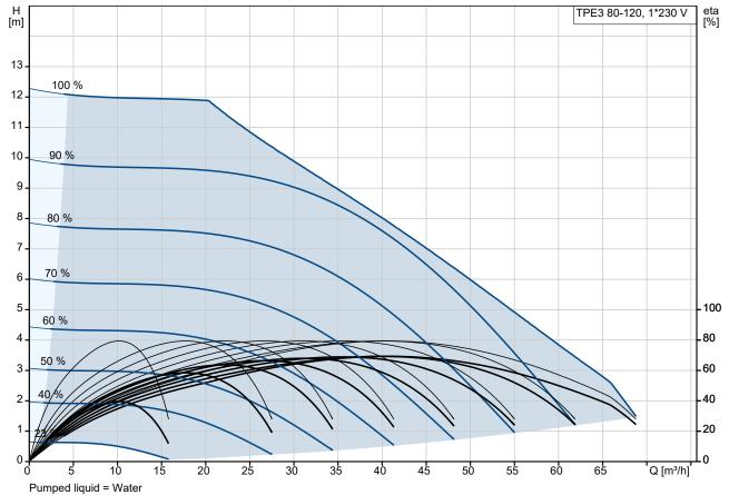
Liquid temperature during operation = 20 °C
