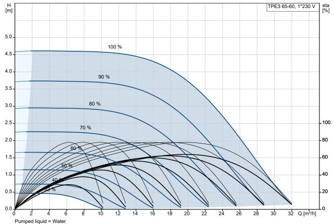
Liquid temperature during operation = 20 °C Density = 998.2 kg/m³
