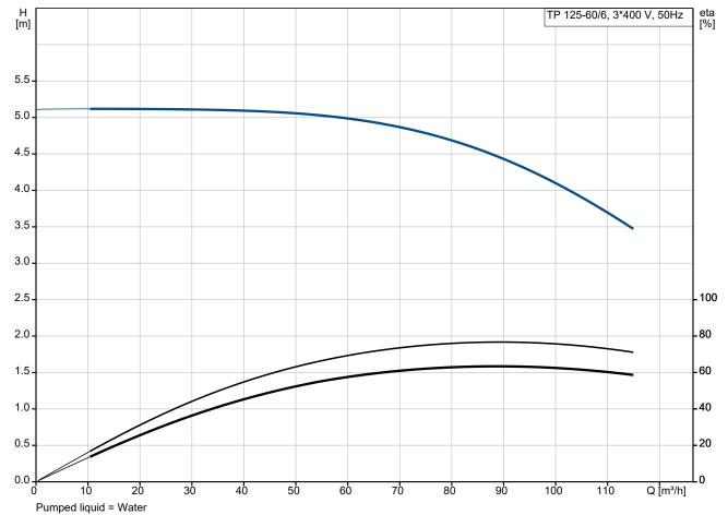
Liquid temperature during operation = 20 °C
