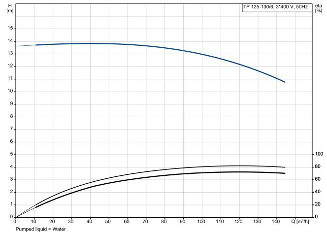
Liquid temperature during operation = 20 °C Density = 998.2 kg/m<sup>3</sup>
