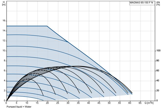
Liquid temperature during operation = 60 °C Density = 983.2 kg/m<sup>3</sup>
