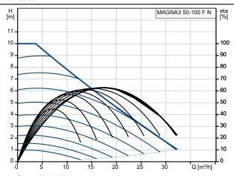
Pumped liquid = Water Liquid temperature during operation = 60 °C Density = 983.2 kg/m³
