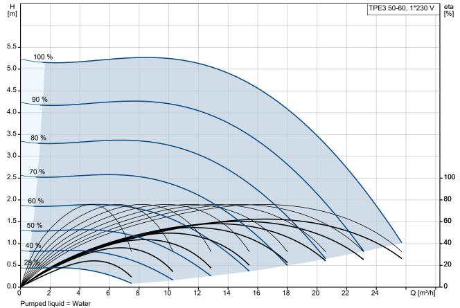
Pumped liquid = Water Liquid temperature during operation = 20 °C
