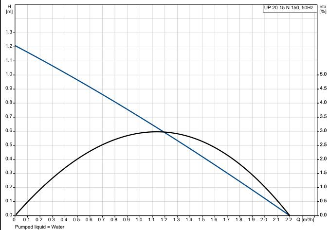
Liquid temperature during operation = 60 °C Density = 983.2 kg/m³
