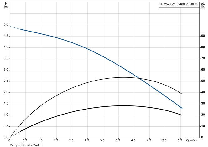
Liquid temperature during operation = 20 °C
