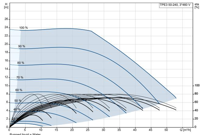
Pumped liquid = Water Liquid temperature during operation = 20 °C Density = 998.2 kg/m³
