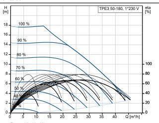
Pumped liquid = Water Liquid temperature during operation = 20 °C Density = 998.2 kg/m³
