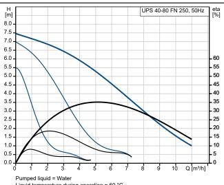
Liquid temperature during operation = 60 °C Density = 983.2 kg/m³
