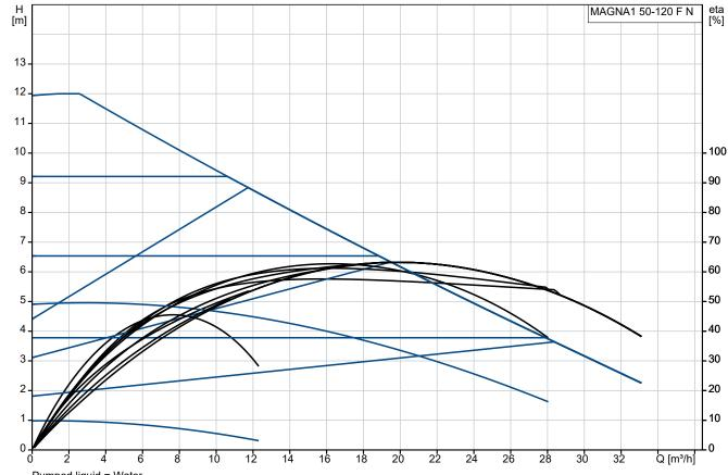
Pumped liquid = Water Liquid temperature during operation = 60 °C Density = 983.2 kg/m³
