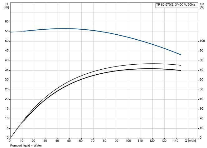
Liquid temperature during operation = 20 °C
