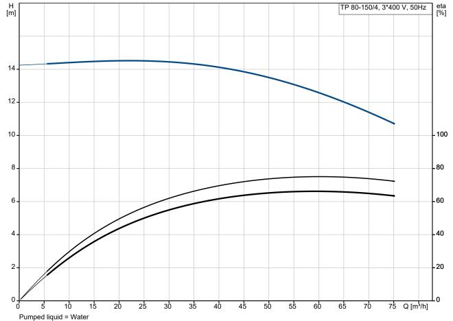
Liquid temperature during operation = 20 °C
