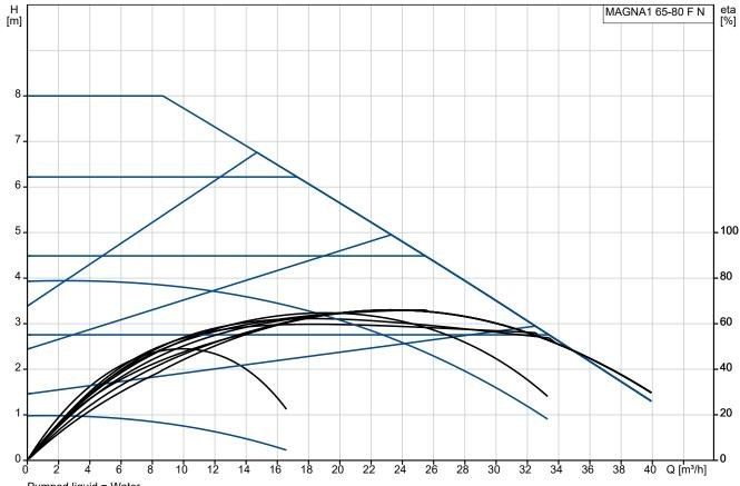
Pumped liquid = Water Liquid temperature during operation = 60 °C
