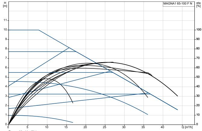
Pumped liquid = Water Liquid temperature during operation = 60 °C
