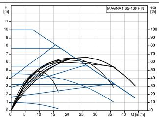
Pumped liquid = Water Liquid temperature during operation = 60  $^{\circ}$ C Density = 983.2 kg/m³
