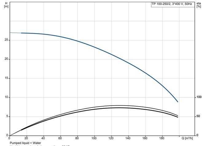
Liquid temperature during operation = 20 °C
